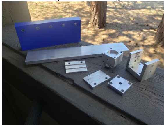
Figure 7: Bracket Clamp Parts and Mock Ring Drill Template
